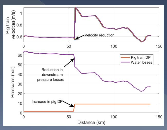
Instead of air pressure building up, upstream – the water pressure drops downstream and the pig train continues without stopping...
